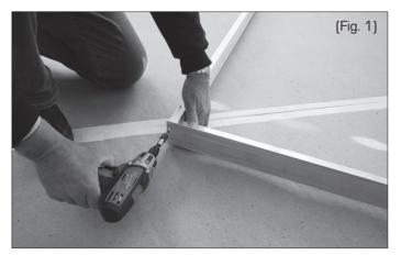
1) Place the sliding door rail and the back board with rubber stopper on a even surface. Fasten the back board to the sliding door rail using 2 pcs of 30 mm screws, H-2. (Fig 1)
